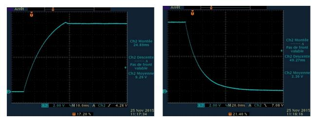
Vo= 12V Io = 2,55 A, Co = 4700  $\mu$ F (CH1), V line = 230 Vac 50 Hz.
